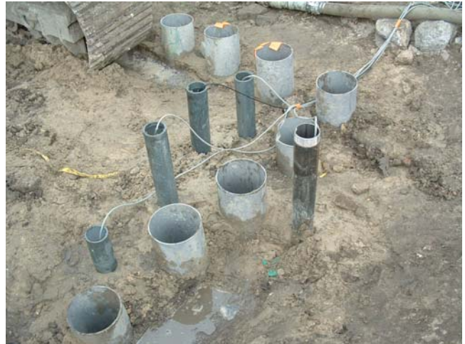
Figure 7 : Hydrophone test setup
