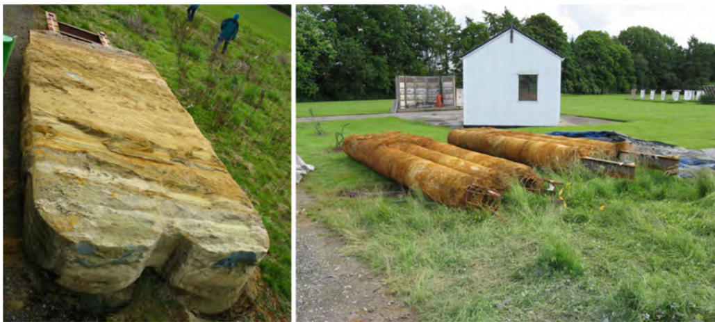
Fig. 6. CSM panels and soil-cement columns before cutting and testing
