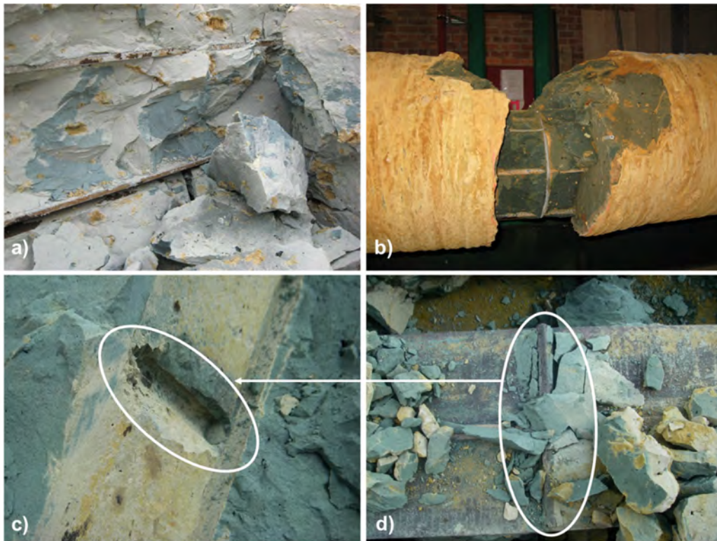
Fig. 13. Soil mix elements after testing and after removal of the steel reinforcement for the half-CSM panel id. 3 (a), the soil-cement column id. 9 (b) and the half-CSM panel id. 6 (c and d)
