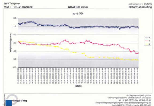
Figure 7: Observed settlements during the installation of micro piles ( z = vertical direction, x and y = horizontal direction)
