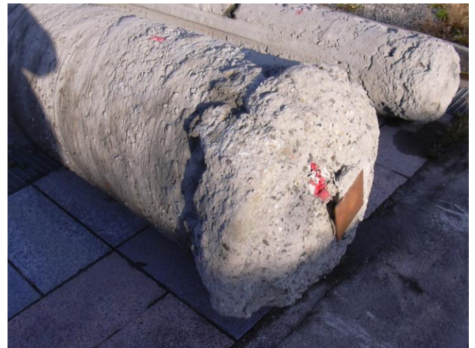
Figure 13 – Excavated CFA pile (left) with casing site Loenhout - detail of the pile base
