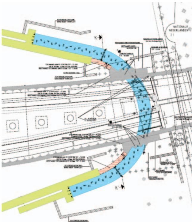
Figure 3. Plan of designed collar construction around the tunnel at station platform elevation, showing frozen soil area (blue) and supporting diaphragm walls (green). Distance between vertical freeze pipes is ca. 0.9 m.
