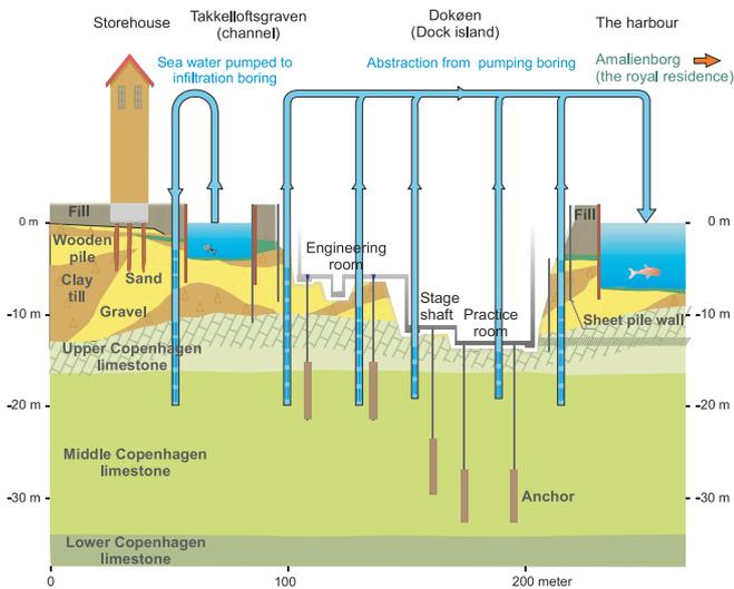
Figure 1. Principal vertical section of the excavation and the groundwater lowering system.
