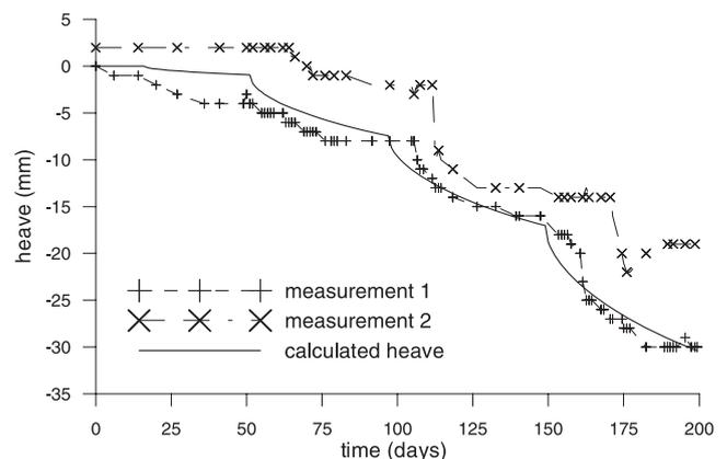
Figure 7. Calculated vs. measured heave (analytical method).
