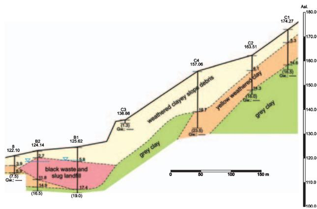
Figure 8. The section of the analysed slope.
