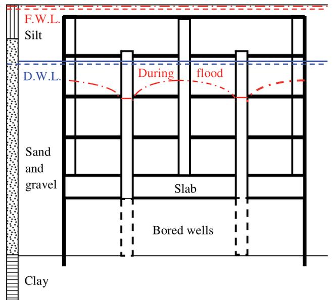
Figure 2. Stability assurance of the Carlton garage for uplift during a flood in the Danube (D.W.L. – design water level, F.W.L. – flood water level).
