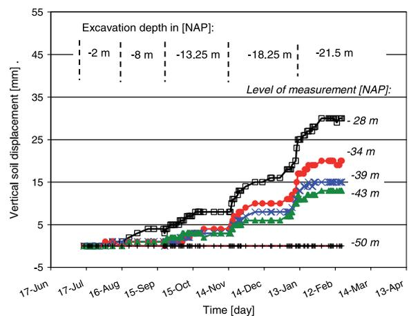
Figure 6. In-situ measurements of extensometers.
