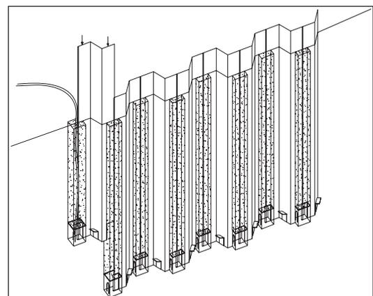
Figure 5. Sheet piling and continuous cement grouting.
