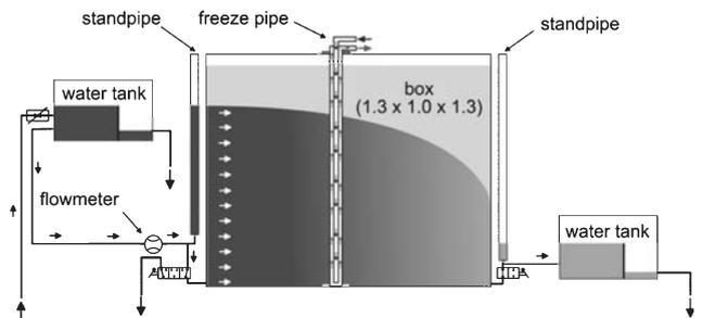
Figure 4. Plan of the large-scale laboratory model.
