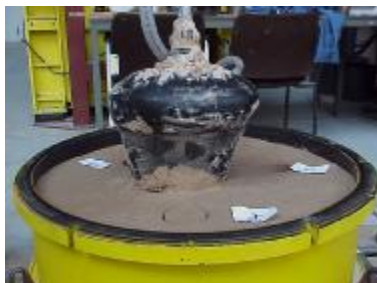
Partly excavated grout body after the test
