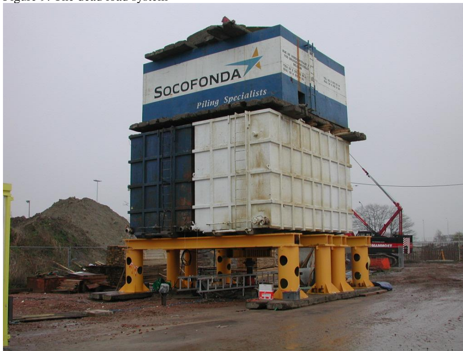
Figure 9: The dead load system
